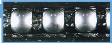
Detail view of the ball cage
